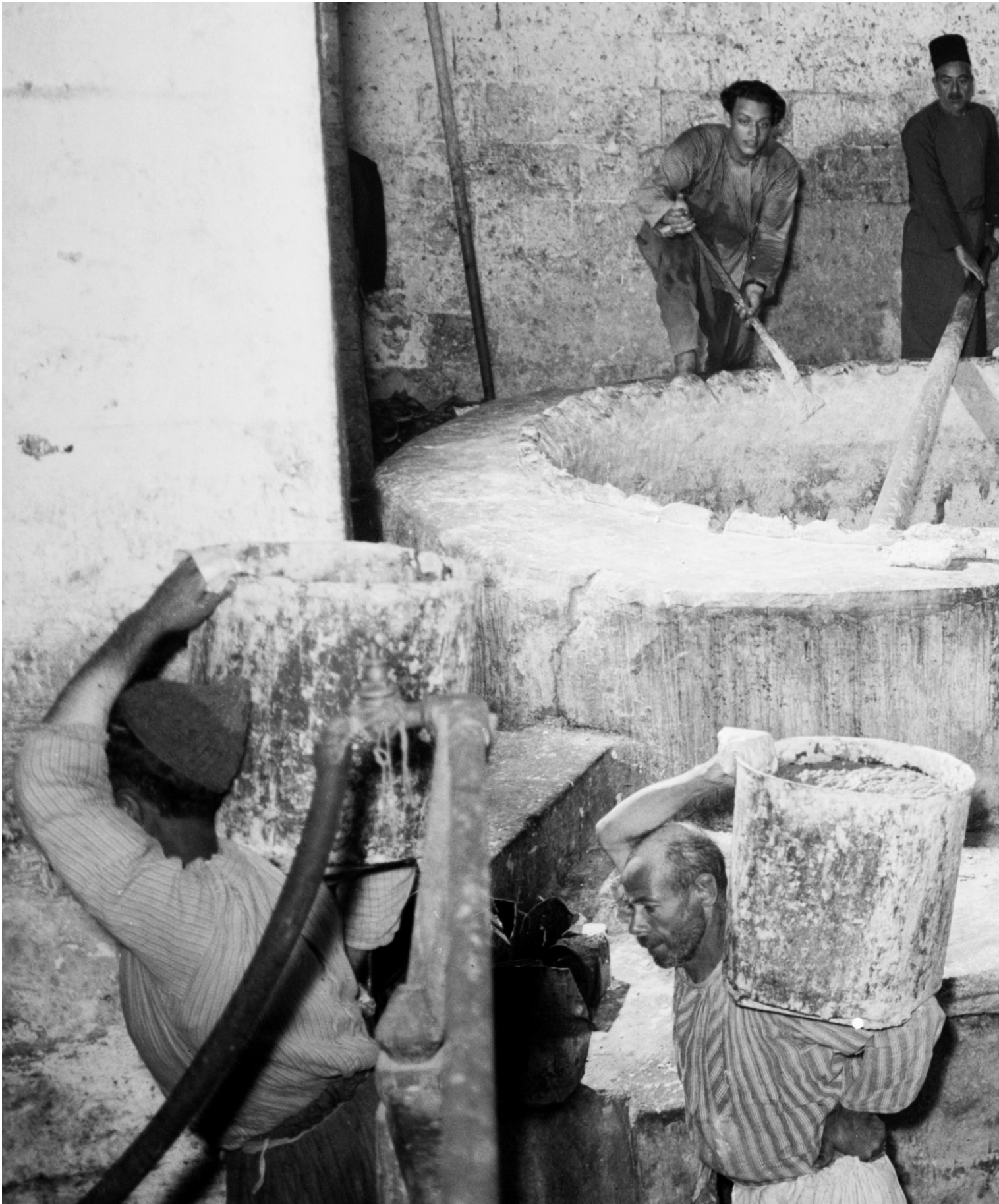
WORKERS LINE UP TO TAKE THE HOT SOAP LIQUID TO THE UPPER FLOOR 104
